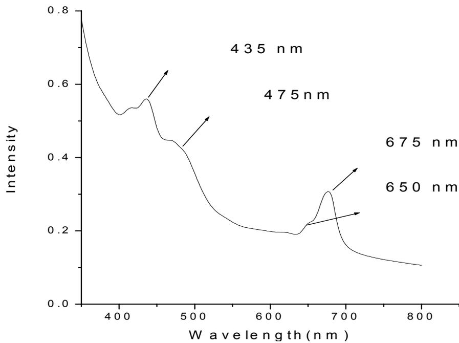
**Fig. 3.** UV-vis absorption spectra of extract in acetone medium.
