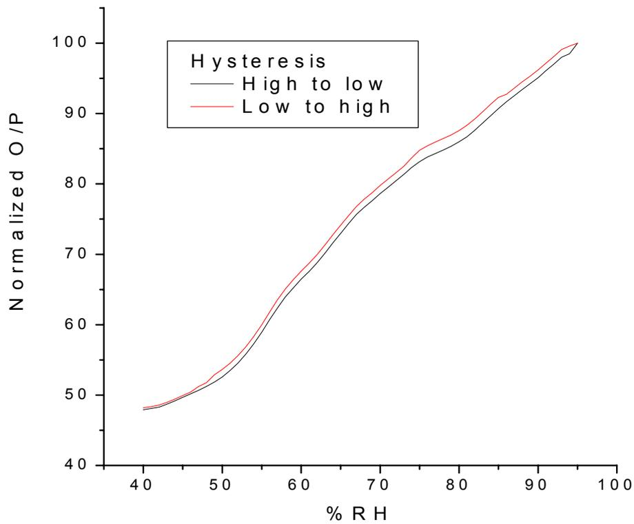
**Fig. 8.** Variation of humidity for increasing and decreasing cycle of a typical sample for 100% concentration, 3mm length.
