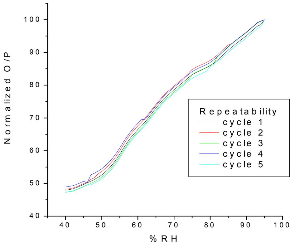
**Fig. 9.** Variation from cycle to cycle of a typical sample for 100% concentration, 3 mm length.
