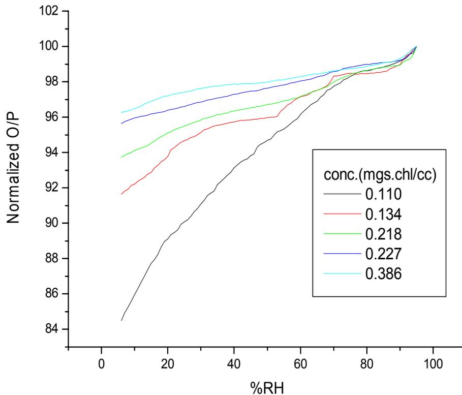
**Fig. 6.** Humidity sensing for clads with different chlorophyll content.
