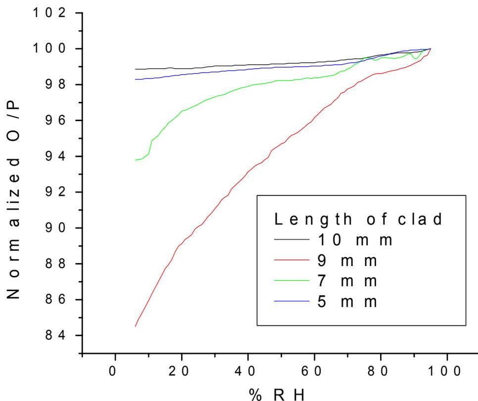
**Fig. 5.** Humidity sensing with variation of clad length.
