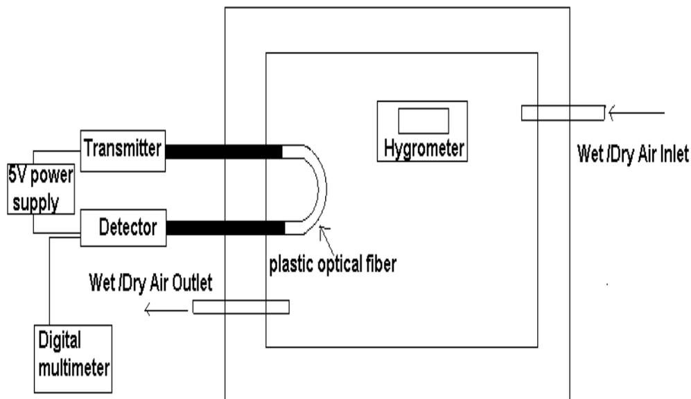
**Fig. 1.** Experimental setup of the sensor characterization system.
