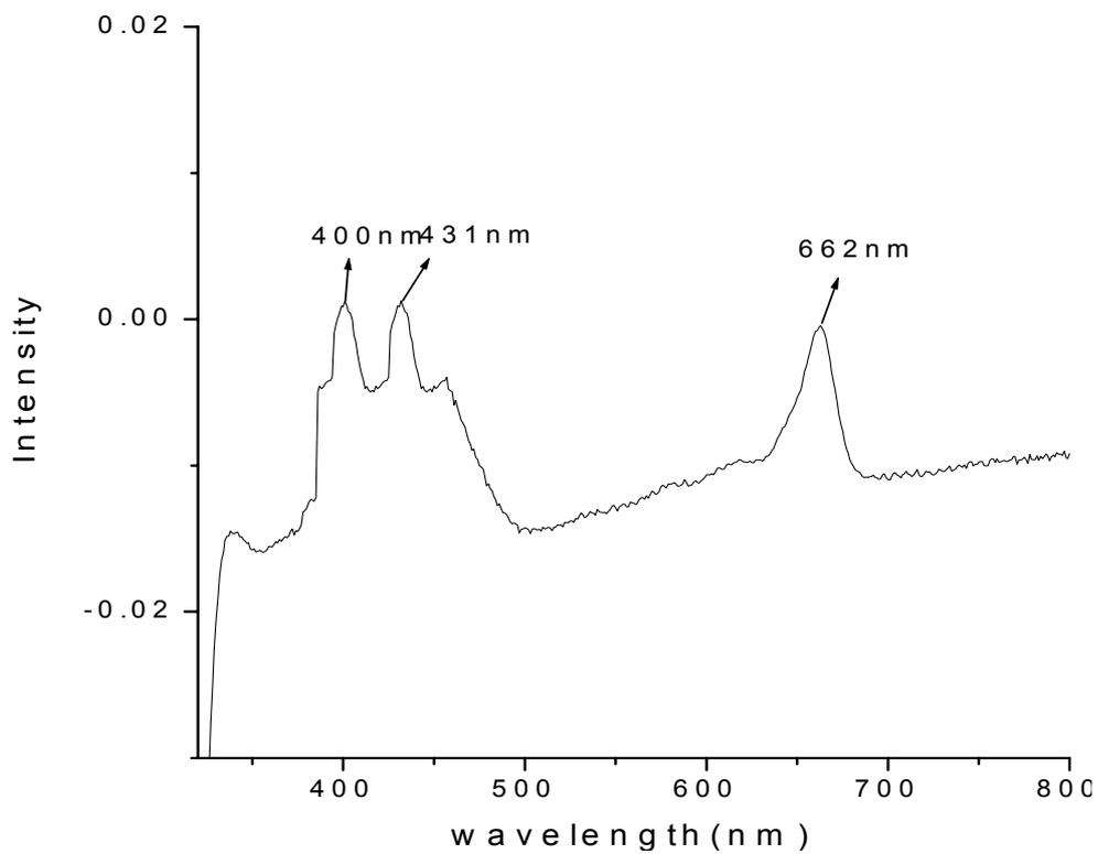
**Fig. 4.** UV-vis absorption spectra of extract with Ag particles in acetone medium.
