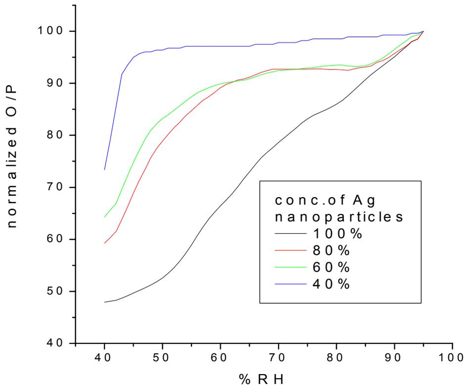
Fig. 7. Response of bio-clad containing different percentages of Ag nanoparticles to humidity.
