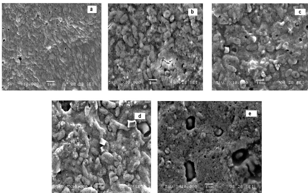
**Fig. 2.** Scanning electron micrographs of films with decreasing chlorophyll content (i.e. 0.386, 0.227, 0.218, 0.134 and 0.110. mgs.chl/cc).
