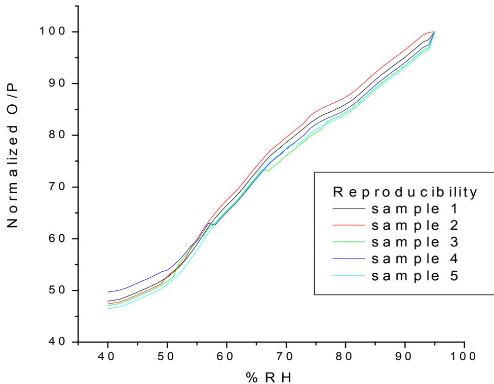
**Fig. 10.** Variation from sample to sample of a typical sample for 100% concentration, 3mm length.
